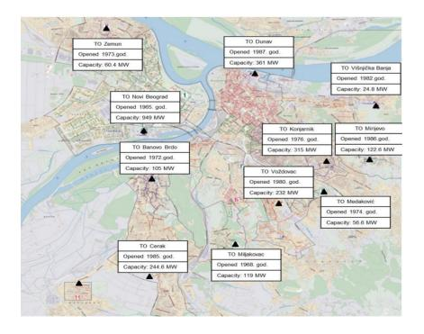
Figure 1: Capacity and location of the main central plants of the Belgrade DH (Source: BE Management and Deloitte analysis).
