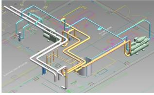
Figure 4. Heat recovery of CHP layout
