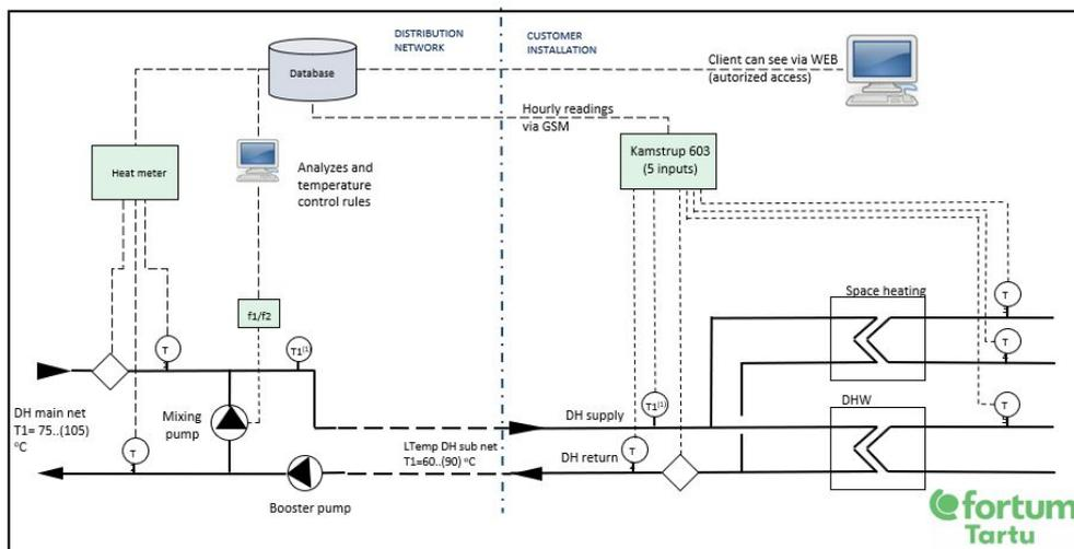
**Figure 2. Technical concept of measuring and mixing system of demo area**
