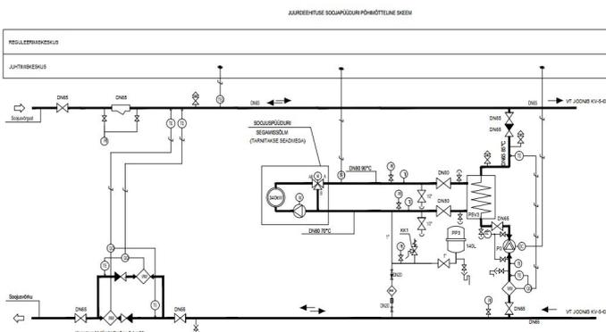
**Figure 3.** Heat recovery of printing house scheme
