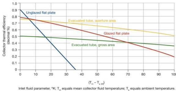
**Figure 1. Thermal performance of collectors vs (Tm-Ta).  $G_T = 800W/m^2$ . Source: Stickney, B. & Soifer, B. (2009).**
