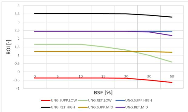
Figure 3. ROI vs Building Solar Fraction for district scale
