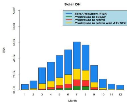
Figure 2. Solar radiation and production for different connection schemes
