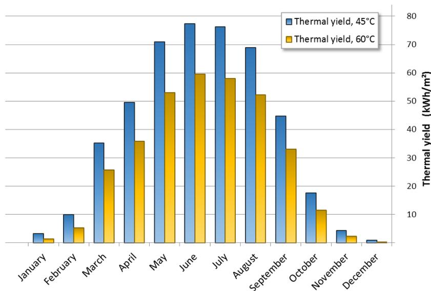
Figure 2 thermal yield for solar collector in Stockholm at 60°C and 45°C respectively.
