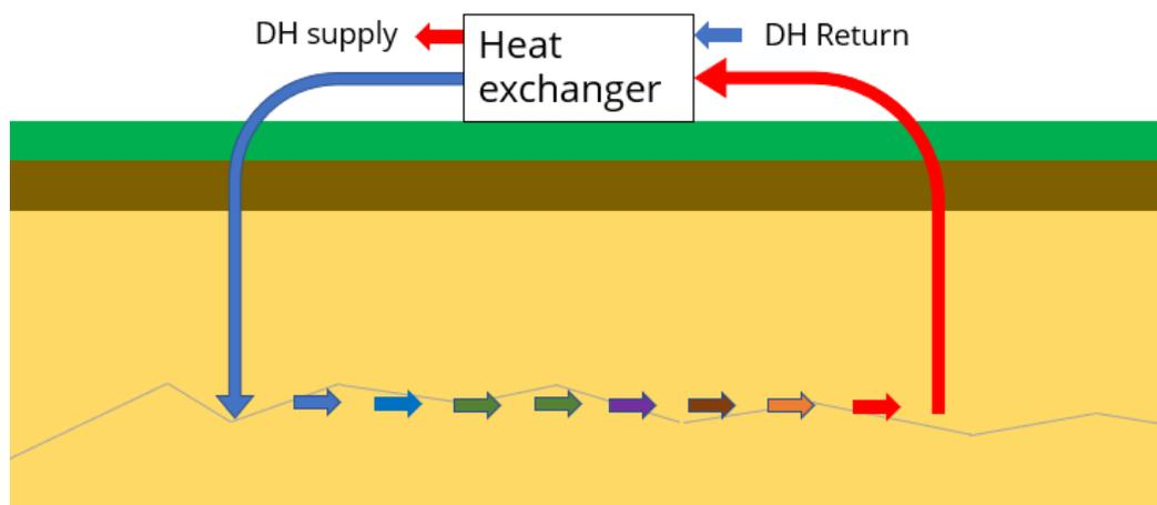
Figure 6 principle of geothermal heat in a DH system
