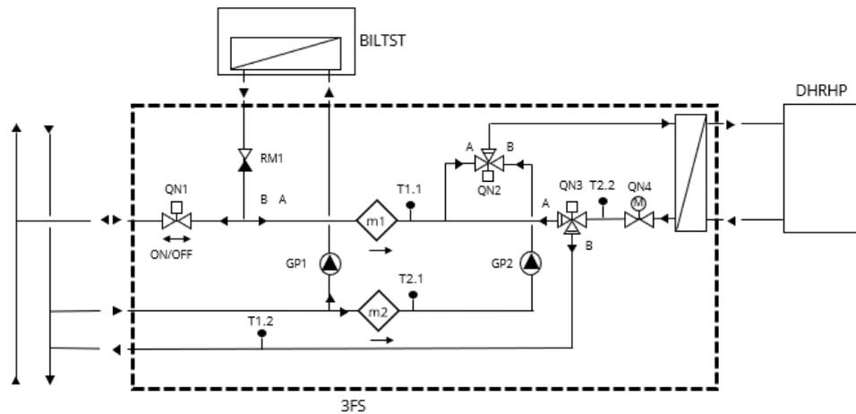
Figure 133. 3FS with DHRHP owned by the building owner and BILTST by the supplier
