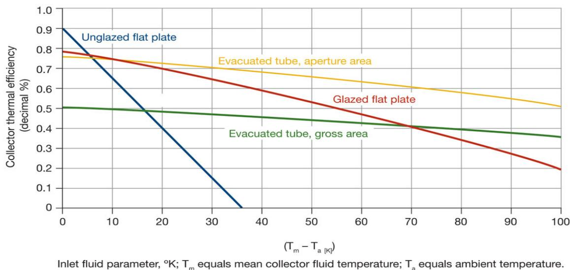
Figure 1: Collector efficiency vs (T<sub>m</sub>-T<sub>a</sub>) [3]
