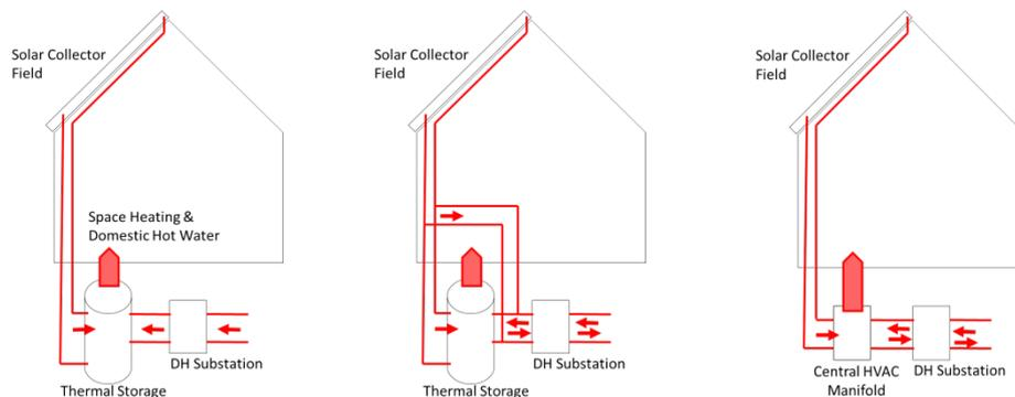
Figure 2: ST integration into DH networks [6]
